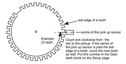
In this example the slot is past the half of the gear. This means that the ECU will fire on coil 2 first and then on coil 1. This setting will be 23 teeth - 18 teeth = 5 teeth and then about 5 degrees for the BTDC setting. For a 60-2 gear the subtract value is 30 instead of 18.
